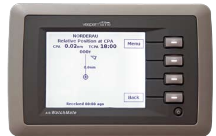
The graphic display here shows that our friend Norderau, on the River Orwell, will pass just 0.02 of a nautical mile away from us in 18 minutes
