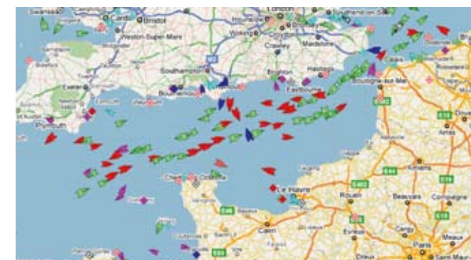
This image from www.marinetraffic.com, a website that follows live AIS transmissions, shows the multitude of ships in the Channel alone and why it is polite for yachtsmen to switch off their own AIS B transmissions in the Solent or other crowded waters
